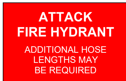
Figure 7 Example of signage required adjacent to external attack fire hydrant
