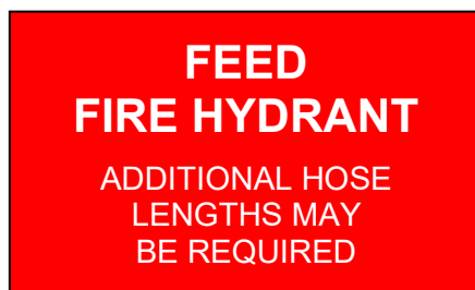
Figure 5 Example of signage required adjacent to each feed fire hydrant
