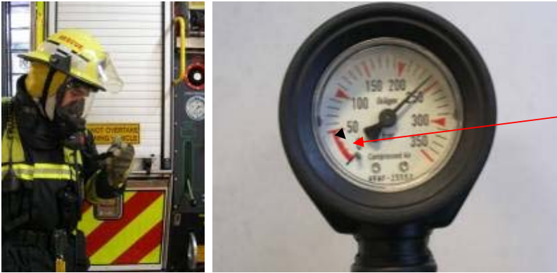
Figure 31 Self-contained breathing apparatus pressure gauge
