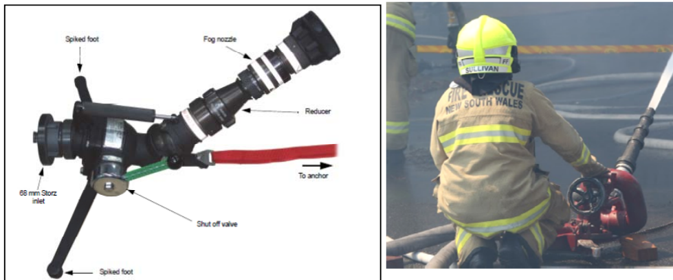
Figure 9 A firefighting monitor
